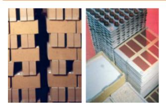
PTCR can be placed at almost any location in the kiln, on kiln furniture, trolleys or transporters. The use of both multilocation and multi-level positioning is recommended, as this provides the most insight into the treatment distribution within the kiln.
